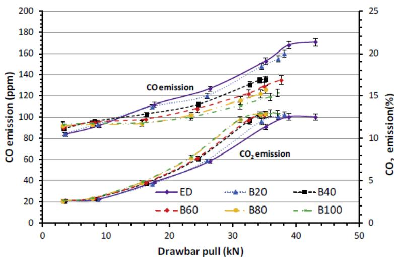
The tests performed in stationary and non-stationary conditions indicated that the changes of engine power, DBP and SFC were statistically highly significant when using B20, B40, B60, B80 and B100 fuels compared to ED. The only exception was B20 blend which use did not show statistically significant difference in engine power with respect to ED during the tests performed in stationary conditions.
