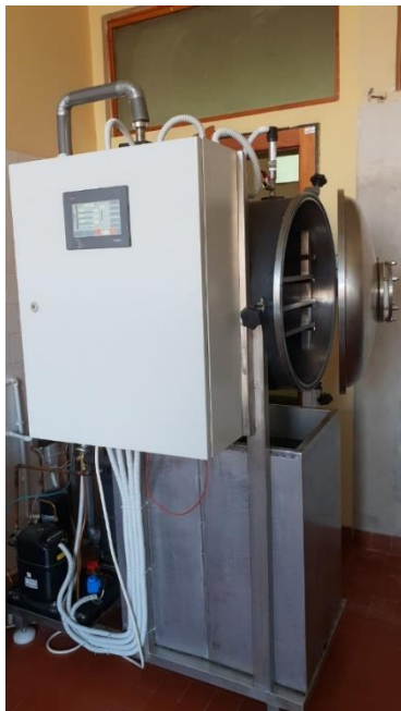
Figure 1. Vacuum dryer with ejector system
